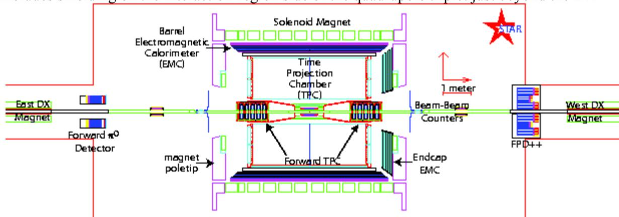
**Figure 9** Schematic layout of STAR in its configuration for RHIC run 6. The FPD++ is an engineering test of a Forward Meson Spectrometer planned to replace it for RHIC run 7. The FMS will provide  $2\pi$  azimuthal coverage in the forward direction, thereby providing STAR with nearly hermetic calorimetric coverage in the interval  $-1 < \eta < 4$ .
