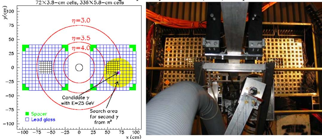
**Figure 10** (Left) Schematic view of the STAR FPD++ as seen from the interaction point looking to the west. The calorimeter size is matched to the requirements for discriminating prompt photons from photon daughters of neutral mesons. The yellow shaded region corresponds to 95% of the decay phase space for  $\pi^0$  produced at large rapidity. (Right) The STAR FPD++ in its configuration for RHIC run 6.
