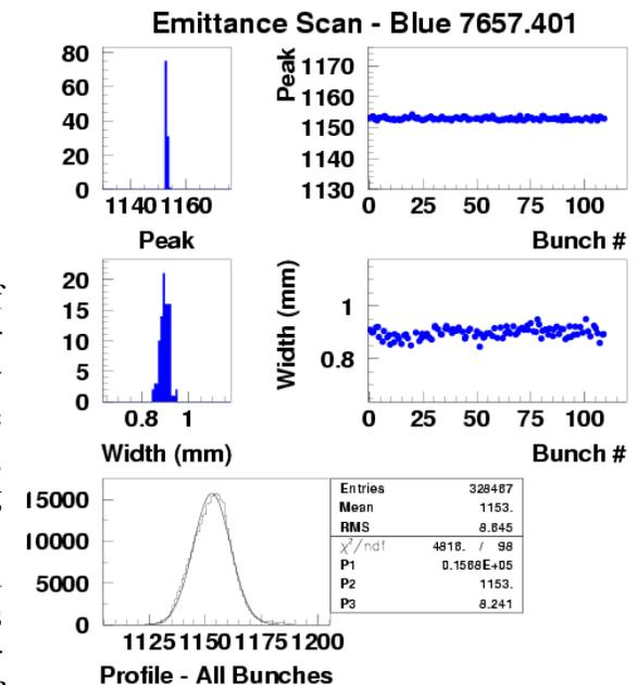
**Figure 18** Measurements with the pC polarimeter that determine the emittance of the RHIC beams via a scan of the carbon ribbon target across the beam. Systematic bunch-to-bunch variations in the emittance are observed.
