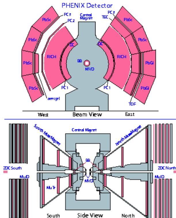
**Figure 13** Plan and side views of the PHENIX
