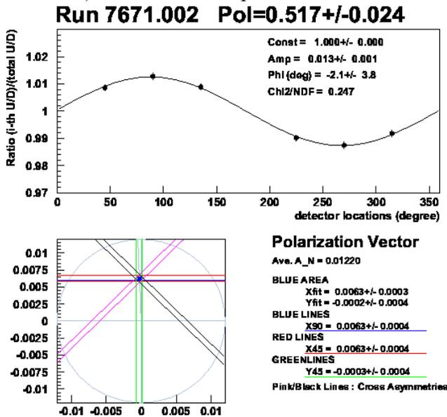
**Figure 17** Raw asymmetries versus detector location (azimuthal angle) measured by pC polarimeter. Fits to the amplitude and phase of the harmonic modulation determine the vertical and radial polarization components of the beam.
